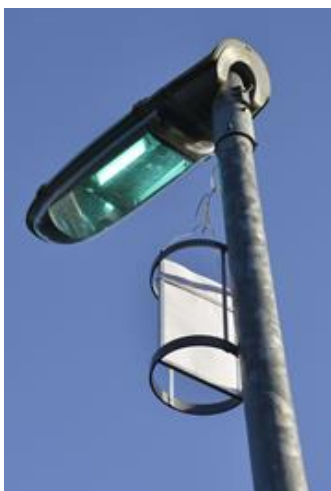
Figure S3: position of custom-made white sticky traps below the light post.
